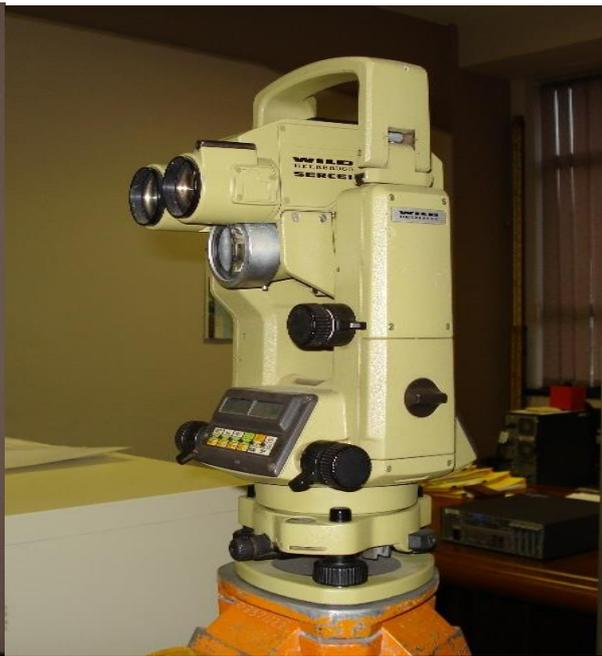
Figure 7 (Theodolite with the EDM attached)
