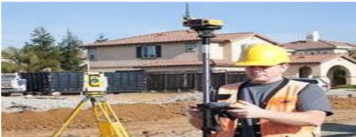
Figure 9 (Robotic Total Station)
