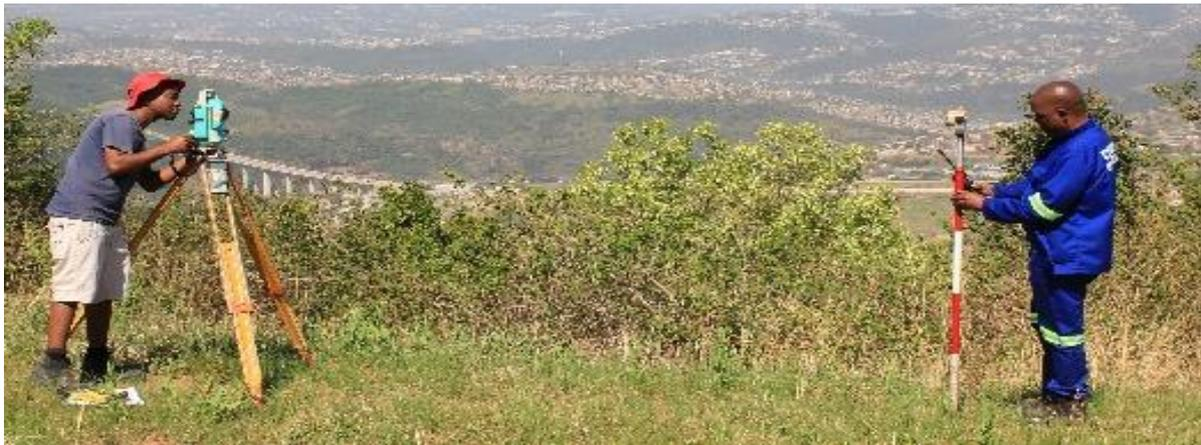
Figure 8 (Total Station – measuring to a prism)
