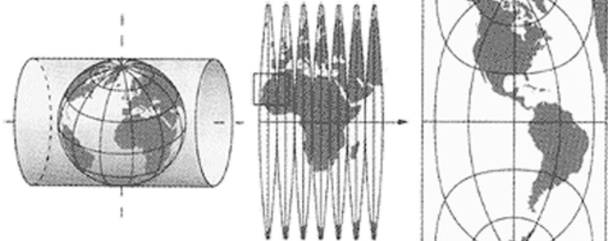
This is an internationally used projection system. The globe is divided into sixty zones each 6° wide. The imaginary cylinder is progressively positioned over the mid point of each zone to create a series of coordinate systems. There is still a bit of distortion so a scale factor is applied to all calculations to try and minimize this.
