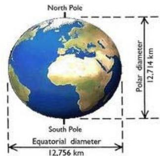
Once an ellipsoid has been defined, lines of latitude and longitude can be generated for that ellipsoid.
