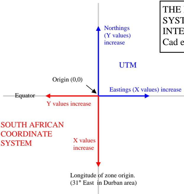
International software such as the ESRI products (ArcGIS etc) and AutoDesk products (AutoCad etc) interpret coordinate values in Universal Transverse Mercator (UTM) orientation as shown in blue to the left. UTM values are referred to as Eastings and Northings (X's & Y's).
