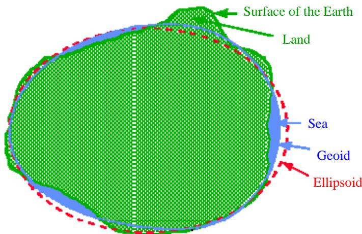
Mathematicians need to define a theoretical surface on which to base calculations. The figure most commonly used is the ellipsoid (imagine a sphere which has been flattened at the poles). This is represented on the figure to the left by a red dotted line.
