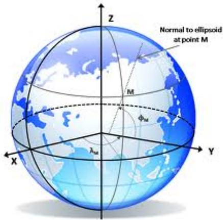
It is important to note that values of latitude & longitude are angles subtended from the centre of the defined ellipsoid and as such are complicated to work with for survey calculations. The vast majority of maps and plans are two dimensional and what is needed are values which define two dimensional position - for example values of Y and X.
